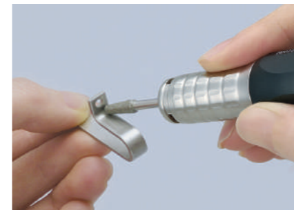
Tool : Electroplated Diamond Burs
